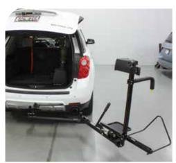
Swing-Away: Rotates the Back-Saver nearly 180° to easily access the hatch, trunk or tailgate.
